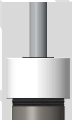
16. Gently press plunger shaft down, while rotating slightly, to insert the seal into the cylinder.
